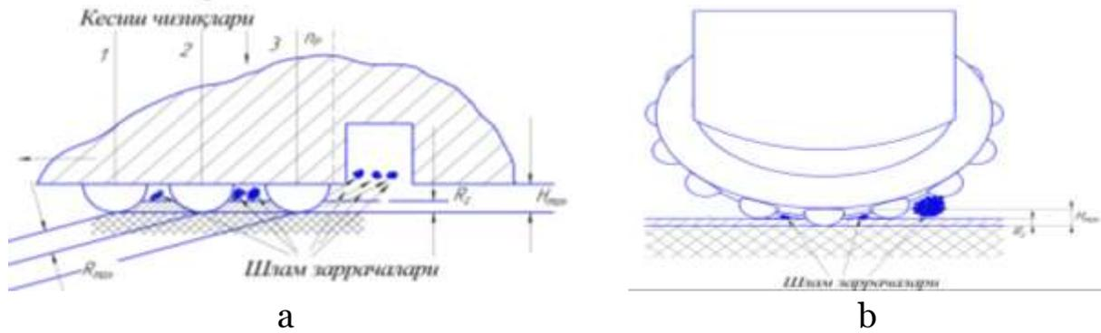
Fig. 1 The movement of sludge particles under the body of the diamond-toothed crown and the spherical dolota and between the teeth.
