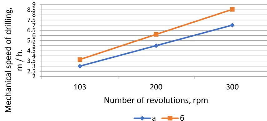
4- Picture. Dependence of the mechanical speed of drilling on the number of revolutions of the drill.
