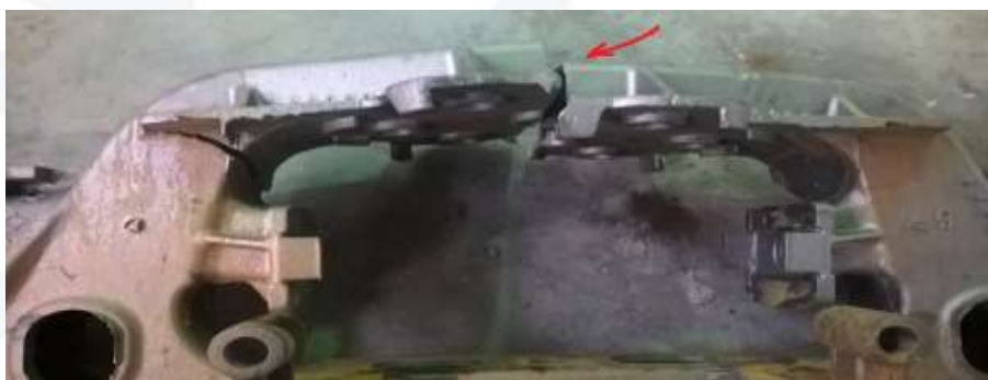
Figure 3 – Side frame break
