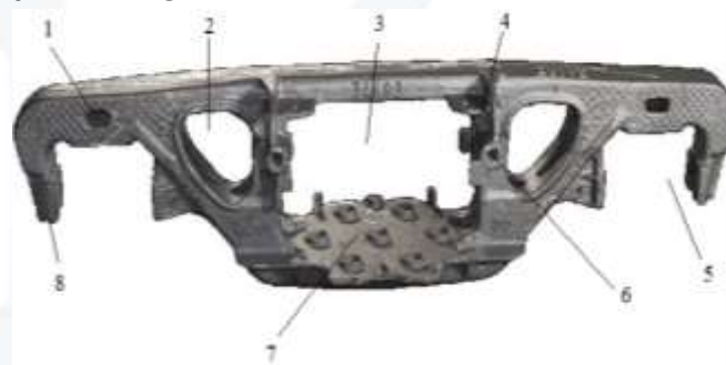
Figure 2 – General view of the part side frame of the trolley model 18-100:
