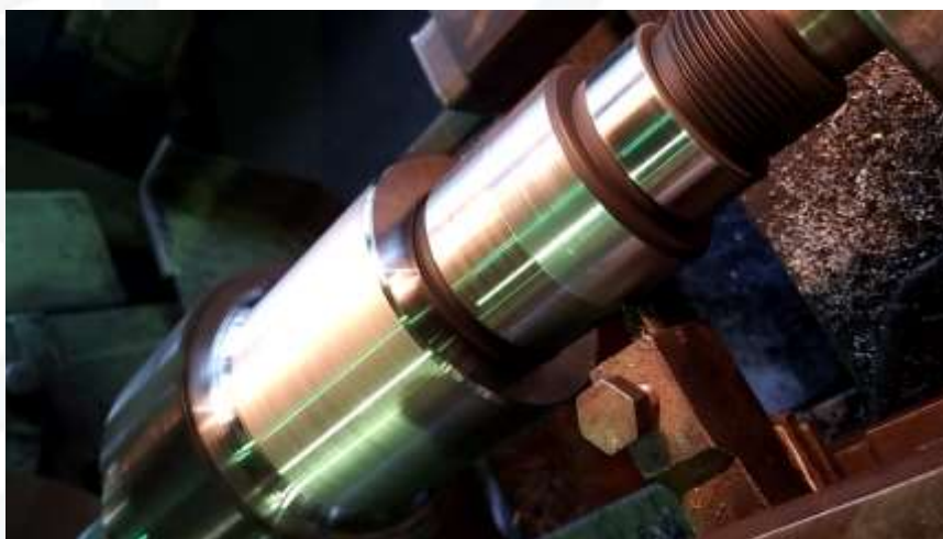
Figure 7 - External longitudinal turning of a shaft made of hardened steel grade 12CrNi3A with a cutter made of tool material based on the B-N-Al- Ti system
