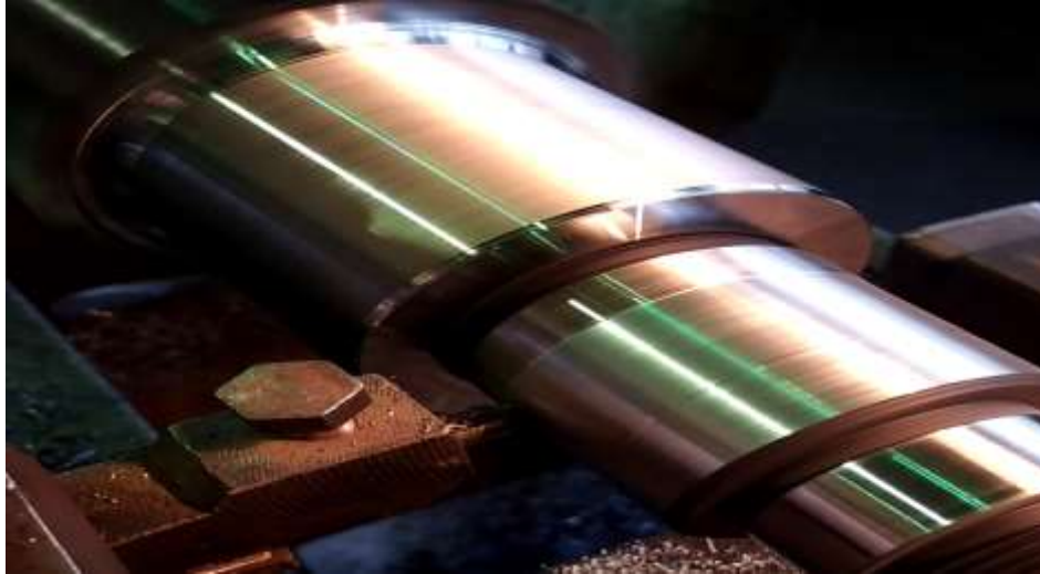
Figure 8 - External longitudinal turning of a shaft made of hardened steel grade 12CrNi3A with a cutter made of tool material based on the B-N-Al- Ti system
