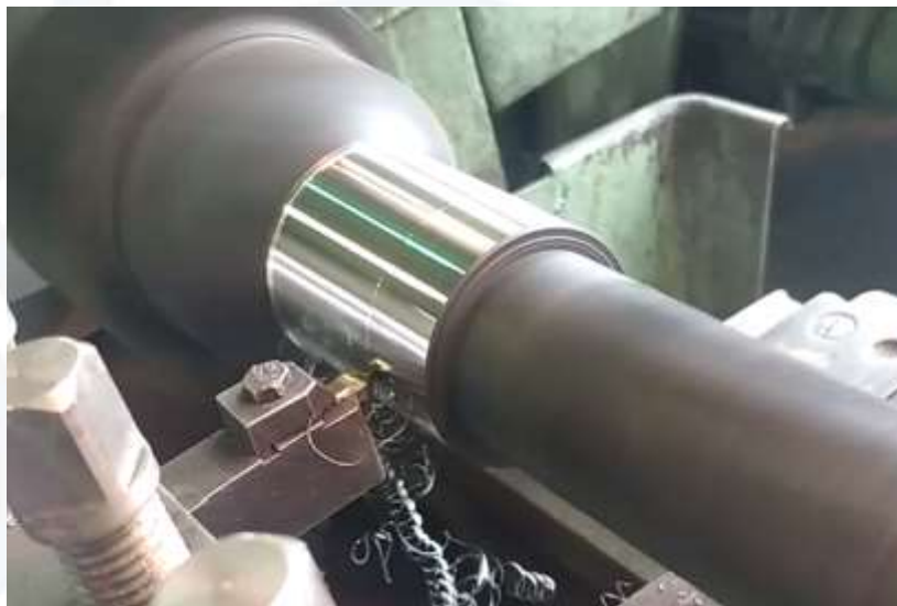
Figure 9. External longitudinal turning of a shaft made of hardened steel grade 12CrNi3A with a cutter made of tool material based on the B-N-Al- Ti system
