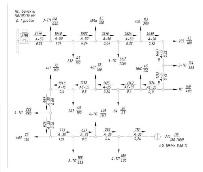
If we use AC-50 wires instead of A-50 wires in the network, we can determine the voltage drop in the network using the above data, where we can see that the voltage drop is DU10kV = 9.79%.
