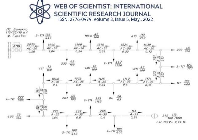
The voltage loss in the supply when using a straight A-50 wire is lower than the mains voltage loss when using an AC-50 wire, but the difference is not significant, but the mechanical strength of the AC-50 wire is A- It differs sharply from the mechanical strength of 50-wire, ie the breaking strength of AC-50/8 steel-aluminum wire is 17112 Newtons, while the breaking strength of A-50 aluminum wire is 8198 Newtons, which means that the mechanical strength of AC-50 wire is more than twice [6].
