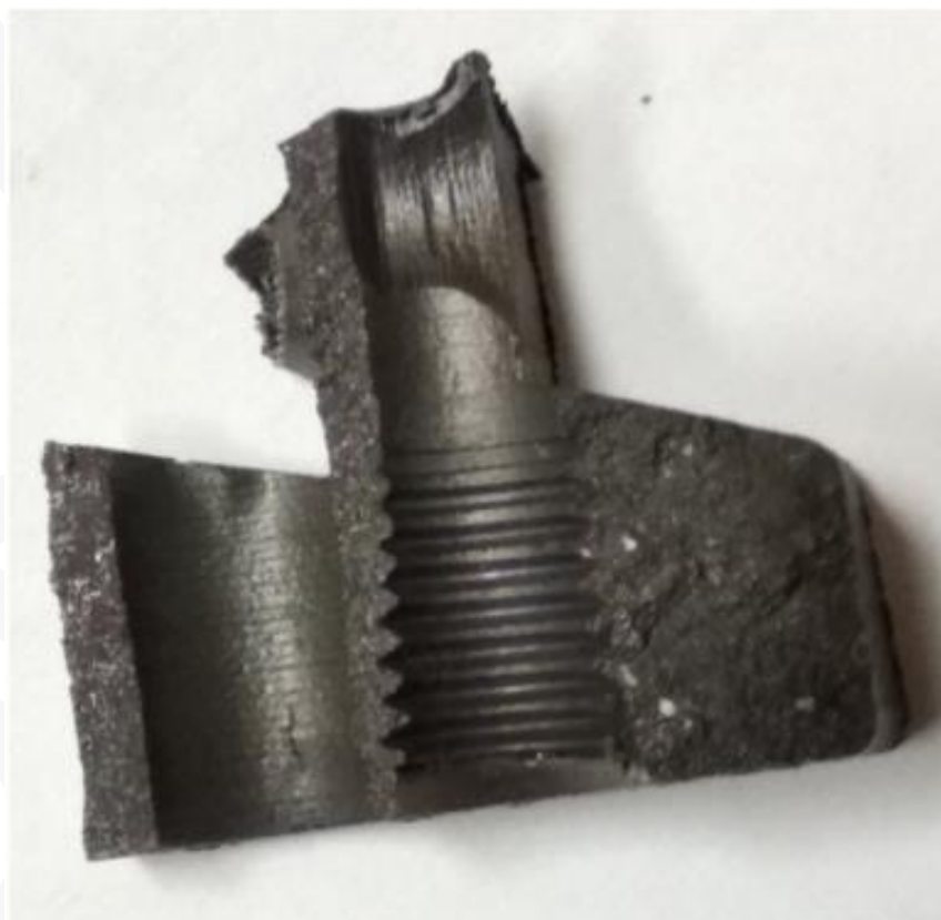
Figure 3. Fracture of the oxidized surface
