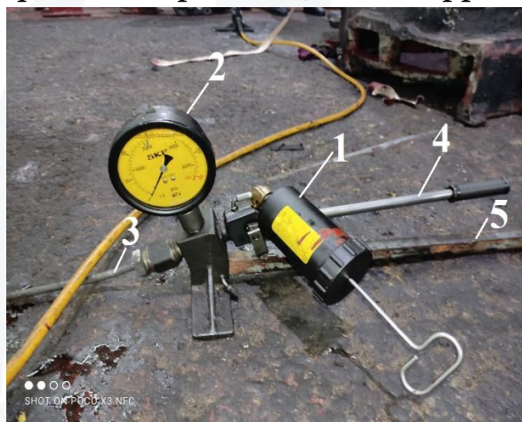
Figure 2. a) gear cold pressing device, b) connecting the tube of the pressing device to the cylindrical support.
