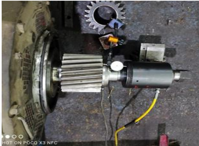
Figure 3. The process of cold fitting the gear to the rotor shaft
