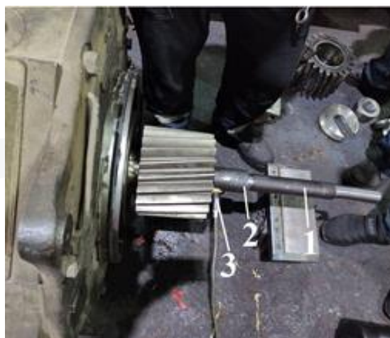
Figure 2. a) gear cold pressing device, b) connecting the tube of the pressing device to the cylindrical support.
