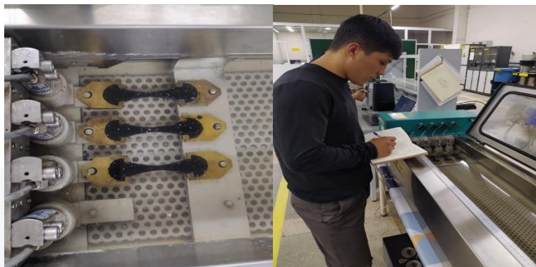
Figure 2. Bitumen flexibility determination
