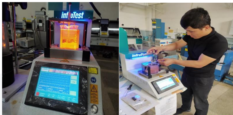
Fig. 3 Determination of softening temperature of bitumen
