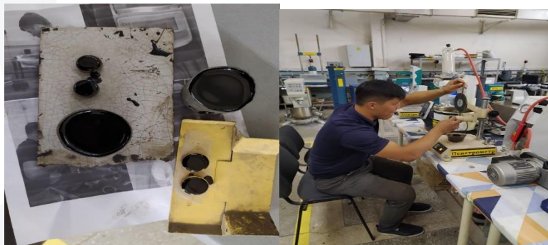
Figure 1 Determination of conditional viscosity of bitumen
