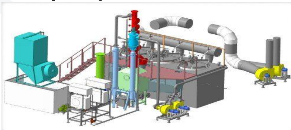
Figure.1. Pirotex - pyrolysis recycling mini-plant for processing of car tires, processing of plastics, polyethylene and rubber
