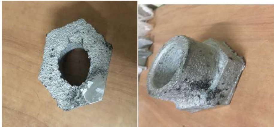
Figure 5. Casting the socket with sand.
