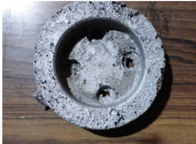
Figure 8. Casting the coupling with sand.
