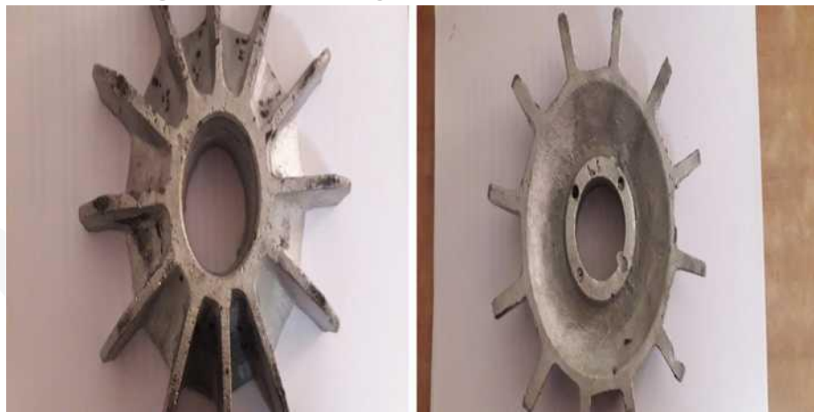
Fig. 6. Casting the propeller with sand.
