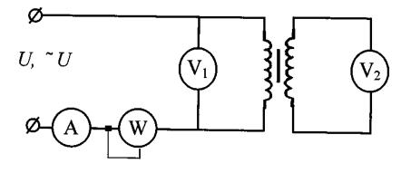
Electrical data for scheme-2 : S<sub>H</sub>uo03d 15 k B · A - transformer power; U<sub>1</sub>uo03d 3 V - voltage of the DC network; I<sub>1</sub>uo03d 25 A - ammeter reading at U<sub>1</sub>.
