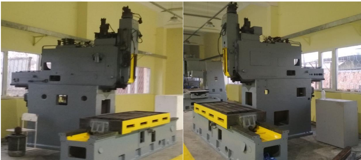
Fig.5. FP-17SMN4 CNC vertical milling machine
