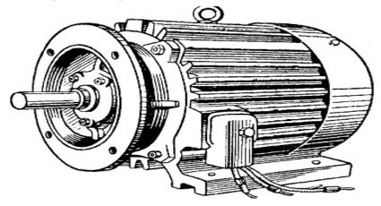
The asynchronous engine is made up of an excitable part — a stator and a rotating part — a rotor. The stator was fitted with a spindle assembled from some electrotechnical steel plate, with three scrolls of copper wire pushed 120° in space into the ditches (pazlaiga) on its surface. The scrolls are attached to a three-phase electrical grid connected by an asterisk or triangle method. The resulting magnetic field of the Stator windings is rotating and crosses the rotor windings.
