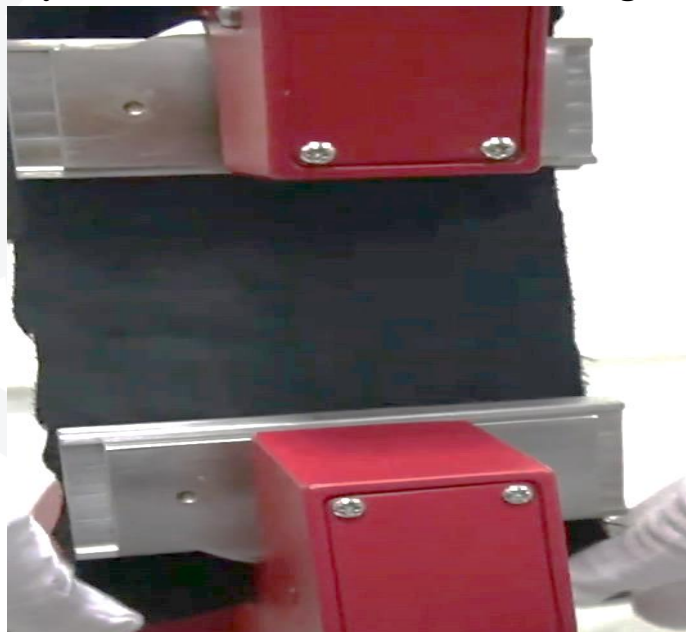
Fig.5 - Tearing of fabric on a tearing machine
