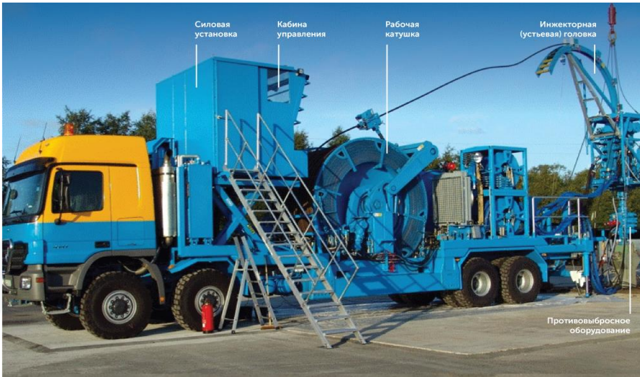
Fig.5. Coiled tubing installation
