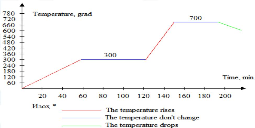
Fig. 3. Primary baking graph of a solid alloy sample.
