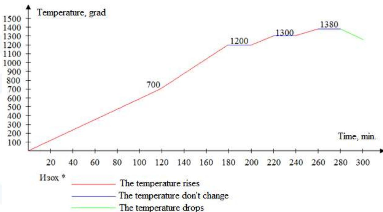
Fig. 4. Baking graph completing the solid alloy sample.
