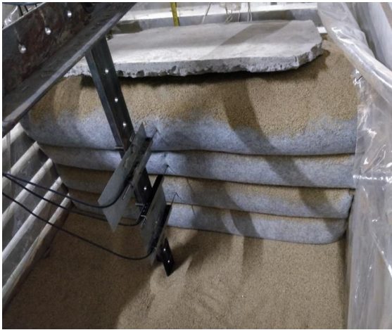
[Fig. 2]. Setting of Setting of displacement sensor.
